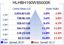
Note: The Curves indicate the illuminated area and the average illumination when the luminaire is at different heights.
