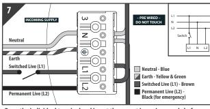
Press the individual terminal and insert the correct incoming supply before releasing the terminal to secure. The product MUST be earthed
