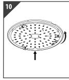
Align gear tray with screws and tighten
