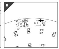
Connect battery pack cable to lamp panel
