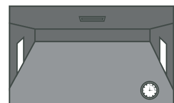
Once the hold time is elapsed, the sensor switches off the light when motion is no longer detected.
